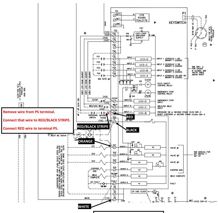
Set DIPswitch 3 (DP3) to the OPEN position. This is the second-stage mode needed to allow the electrodes to open if continuity is not detected.
