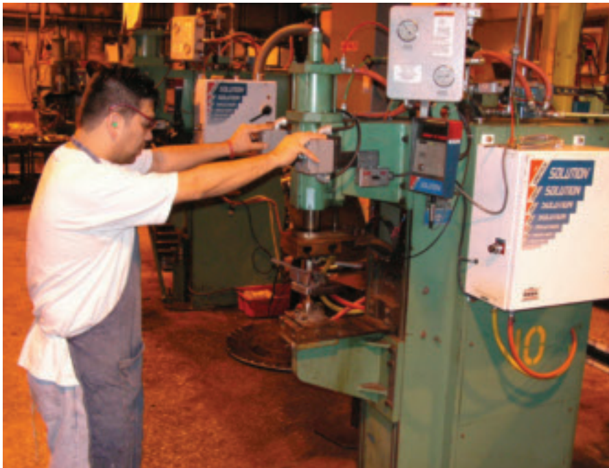
Fig. 4 — Two-hand antitiedown switch welding machine initiation.
