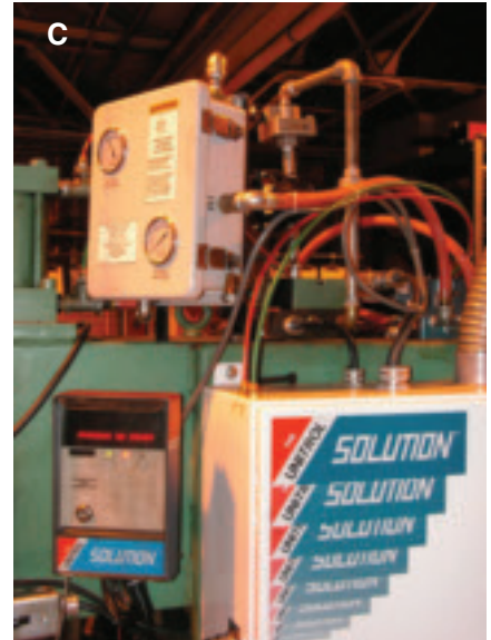
Fig. 6 — A — This system from Unitrol Electronics provides passive electrode pinch-point protection at Ada Metal Products, Inc., Lincolnwood, Ill. B — continuity measuring wires connected to welding transformer secondary pads; C — padlocked NEMA-4 enclosure with precision regulators supply pressure to new solenoid and quick exhaust valves. This arrangement counterbalances an 160-lb ram to less than 40 lb.
