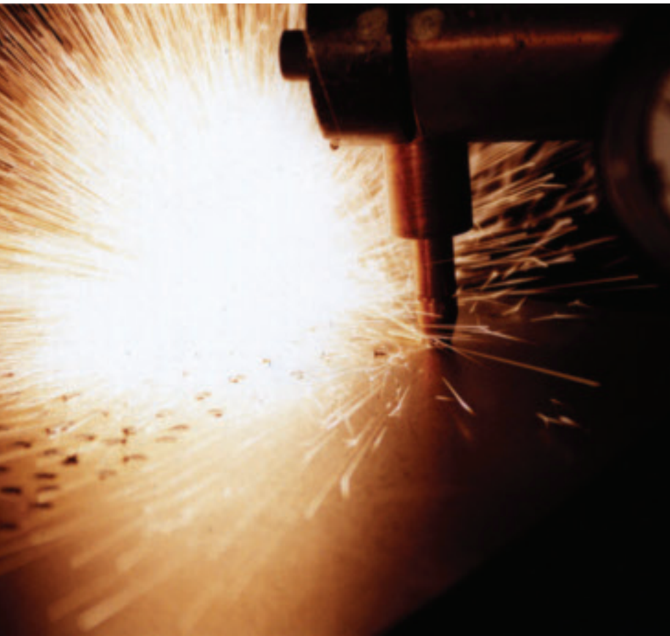
Fig. 1 — Metal expulsion typically caused by low electrode force.
