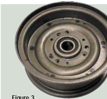
Figure 3 Projection welds replaced 12 rivets on this idler pulley.
